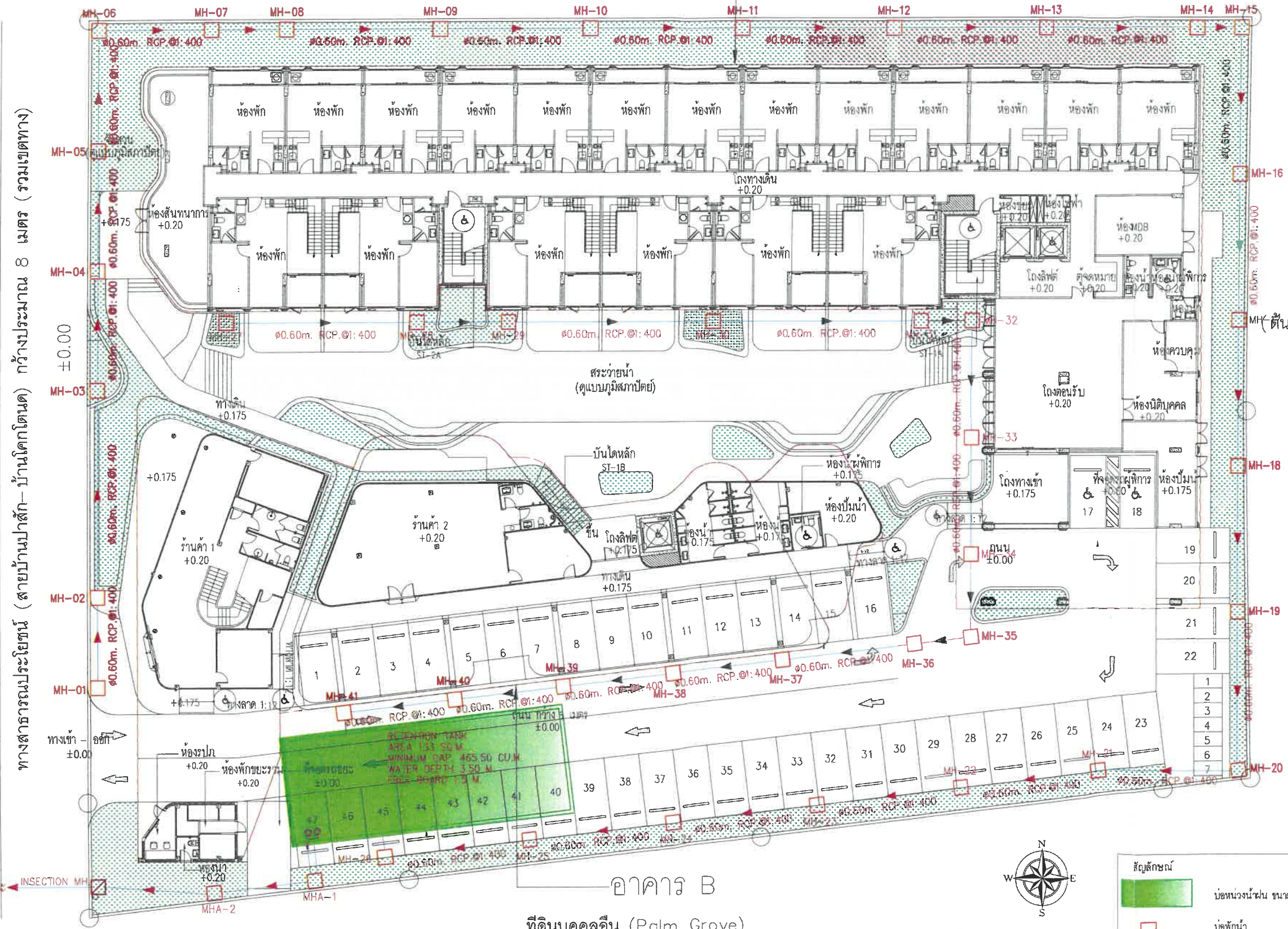
STORM DRAINAGE SYSTEM LAYOUT PLAN SCALE 1:200
